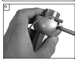
Loosen set screw in half ball, remove pin from downrod and save all parts.
